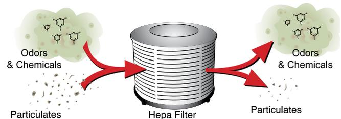
As air passes through a filter, small particles that are floating in the air are trapped. This is helpful in reducing particles such as dust and pollen but is *only part* of the solution. Most gases and odors pass right through even the best HEPA filters.
